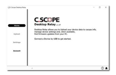
C.Scope Desktop Relay for use with all C.Scope data logging XL4 Cable Avoidance Tools, SGV4-D Signal Generators and MXT4-D Transmitters. Data log upload interface for use with Windows PCs.
