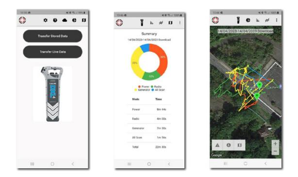
C.Scope Relay App for Android or iOS devices, for use with all C.Scope XL4-DBG GPS and Bluetooth<sup>™</sup> equipped Cable Avoidance Tools.
