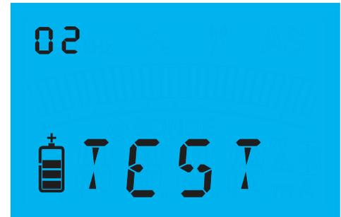
**i** **NOTE** The Locator records every Automatic Daily Self Test. The Test results can be retrieved from the Locator to produce a Product Validation Certificate by using the PC Toolkit (see page 57).
